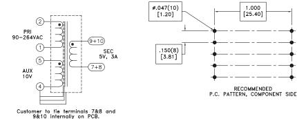
Application of the transformer allows for the leadwires between terminals 7&8 and 9&10 to solder bridge.
